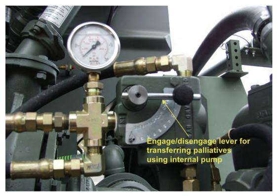
Photo 22. Hydraulic suction pump engagement lever on Finn hydroseeder
