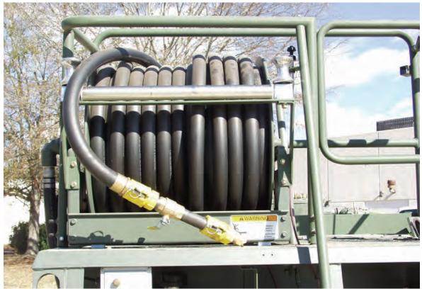
Photo 25. 200-ft hose with electric reel for multiple-use palliative distribution
