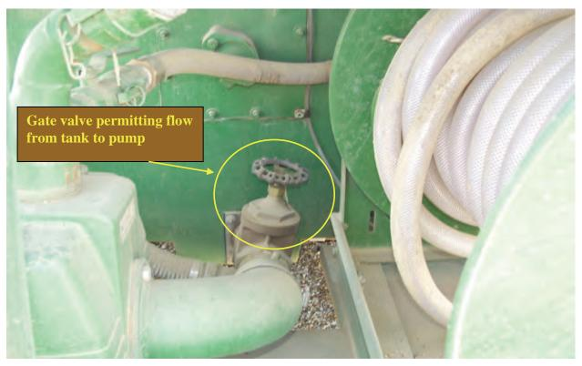
Photo 19. Gate valve on Easy Lawn hydroseeder (must be closed when transferring liquids using onboard pump)
