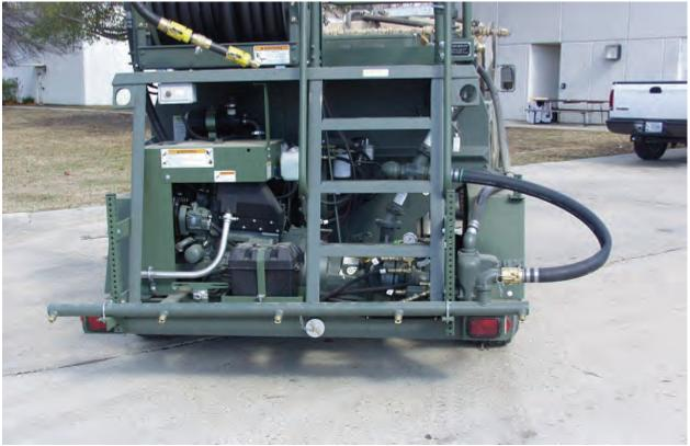
Photo 29. Distribution bar on rear of hydroseeder
