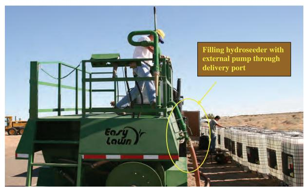
Photo 15. Filling Easy Lawn hydroseeder using external pump
