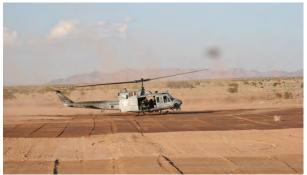
Photo 4. UH-1 landing on helipad treated with synthetic fluid
