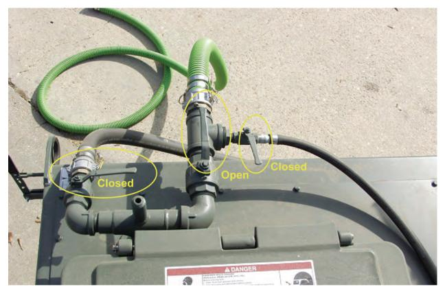
Photo 20. Filling hydroseeder from external pump or water source
