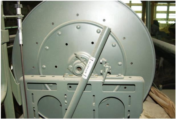
Photo 26. Clutch lever for operating pump
