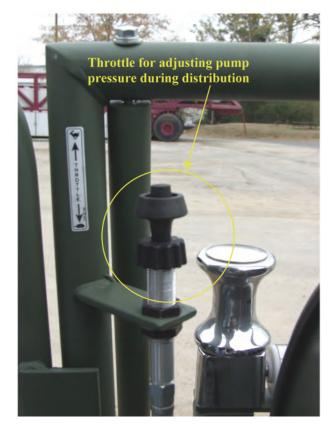
Photo 27. Engine throttle for Finn hydroseeder located by tower gun
