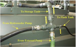
Photo 5. Multiple distribution paths for filling hydroseeder
